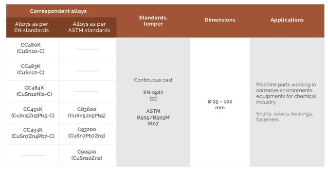
By request, LAROMET can offer vertical continuous cast round bars made of other tin bronzes.
